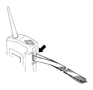
(3) Putting both edges of the strap together, pass it through the openings of the buckle.
